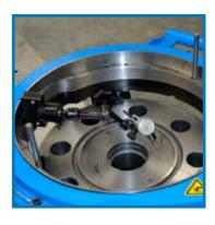
Attach chucking feet to the machine.
