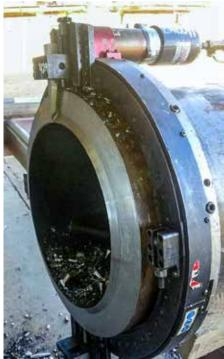
Remove condenser tubes and seal welds with speed and accuracy. This model BR is equipped with our AirLock, pneumatic locking option increasing the speed even more.
