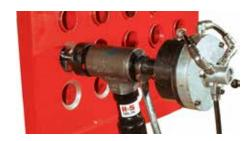
Another compound bevel. This 37.0°-10.0° bevel was placed on a 24.000" (609.6 mm) pipe, 3.500" (88.9 mm) wall in P22 material. It was accomplished in a single machining step with our AFC 24 split frame tool and our resharpenable form tool.
