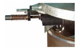
Make short work of stub removal from headers. Here our model MB-110 is equipped with special blades, made to specs, that remove stub weld, chamfer the header and clean up the tube seat in a single pass. Contact us with your specifications to see how easy it is to save time and money.
