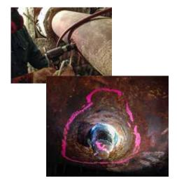
Make fin removal easier and faster. Multi-Prep® features replaceable carbide inserts that will remove 3.500" (88.9 mm) of fins then place a bevel on the tube end in one pass.
