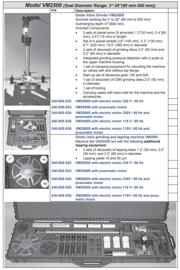
Pneumatically driven machines also require the accessory pneumatic motor maintenance kit
