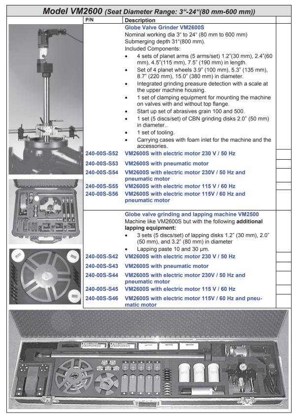
Pneumatically driven machines also require the accessory pneumatic motor maintenance kit
