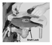
5. Install the blade onto the inside arbor. Place the outside arbor onto the shaft with the internal tabs aligned with the slots in the shaft. Insert the bolt into the shaft and
