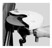
6. Check to ensure that the surrounding area is completely clear. Confirm that the blade is aligned with the cut line. Start the blade disengaged from the panel and slowly push the blade into the panel applying firm, even pressure.
