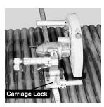
8. In vertical applications, the carriage lock must be used to support the weight of the saw.
