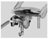
4. Mount the saw power unit/carriage assembly onto the guide rail.
