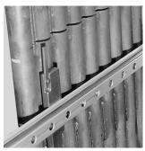
2. Establish your cut line and set the weld tab assembly against the panel. The top of the line indicator must be on the cut line. If the weld tabs are not at a place where they can be welded, remove the tab bolts and
