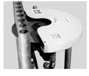
7. Continue cutting until the blade penetrates the wall completely. The TS 400 is a plunge-cut type saw. It is not designed to be pushed along the guide rail in a continuous cutting
