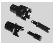
Three types of tube cutters are available - O.D. beveling, water wall membrane removal and an O.D. wall cleaner. All of the cutters are available for tube sizes ranging from 1.25" to 3.0" (31 .8 mm to 76.2 mm) O.D. in .250" (6.3 mm) increments. The tube size is stamped on the cutter.
