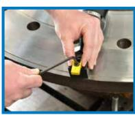
Install tool bit. Connect to power.
