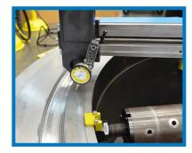
Adjust the turning arm and couterweight arm to the correct diameter.
