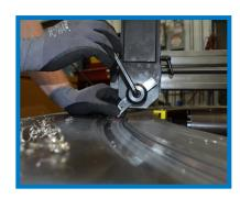
Set machine onto flange using setup fingers.
