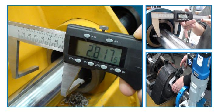
The digital bore measuring caliper features a patented design, allowing you to measure 10 inches (254 mm) or 24 inches (609.6mm) around your line boring equipment. Now you can get an accurate reading of the bore without removing the bar. This precision tool also allows outside measuring, saving you time and money.
