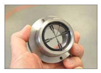
When viewing through the Brunson alignment telescope, the far side target will be distinguished from the near side with the use of a custom designed open wire target. The unique 45° "clocking wire" is easily visible up to distances of 50 feet.
