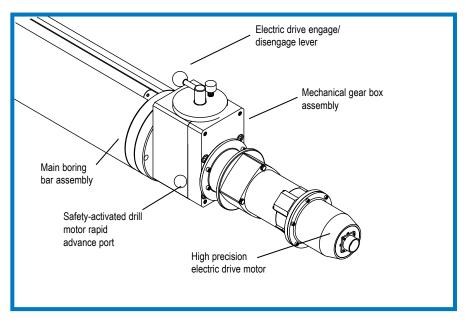
A special adaptor plate allows you to easily connect the electric feed/ mechanical gearbox assembly to Climax 3.5, 5, 6, and 8 inch (88.9, 127, 152.4, and 203.2 mm) boring bars. Adapters are also available for competitive boring systems.
