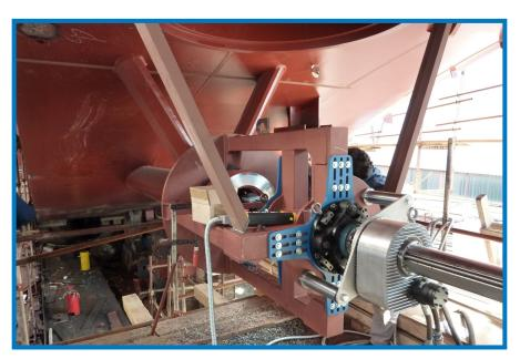
tooling for both boring and facing operations.
