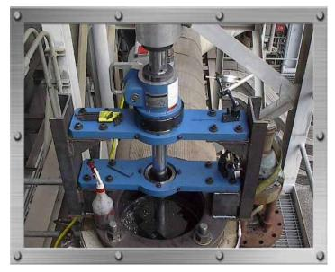
A Cantilever-Mounted BB5000 Boring Machine Performing Valve Repair
