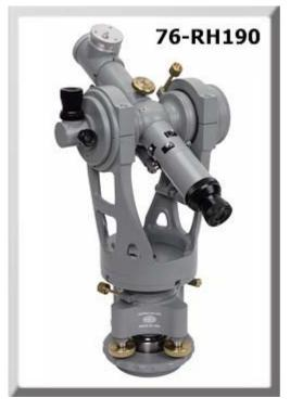
Available with English, metric, or no micrometer. Measurements from the optical reference line are taken by using an optical micrometer mounted on the main telescope. The 76-RH190 comes standard with a model 190 optical micrometer. To order the transit with a metric micrometer, specify 76-RH190M. In event that you do not want either micrometer, order model number 76-RH.
