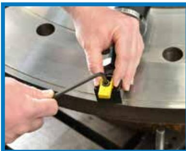
**7** Install tool bit. Connect to power.
