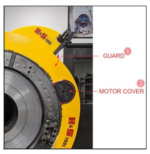
FIGURE 3-1. GUARD AND MOTOR COVER
