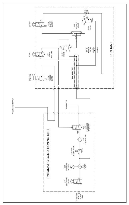
FIGURE B-1. PNEUMATIC CONDITIONING UNIT SCHEMATIC
