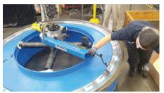
A portable flange facer being used to manufacture a circular mill
